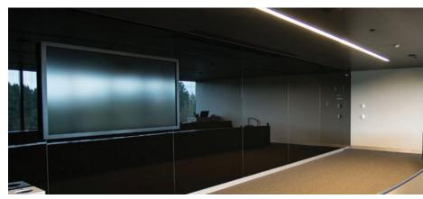
Moon Shadow's largest contribution came by way of the dry-erase glass magnetic boards that serve as writing boards in meeting rooms. Laminated with magnetic properties added to the back, the lites of glass each stand at nearly 9 feet tall and more than 4 feet wide.
